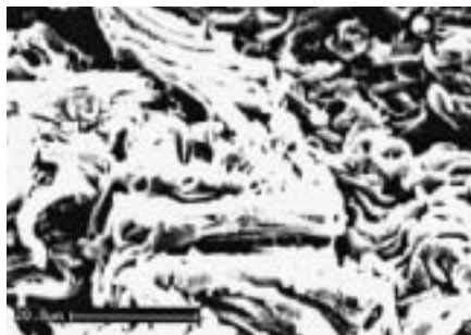
Figure 6a. SEM studies of PP/NR: 70/30 blend without curatives. 107
